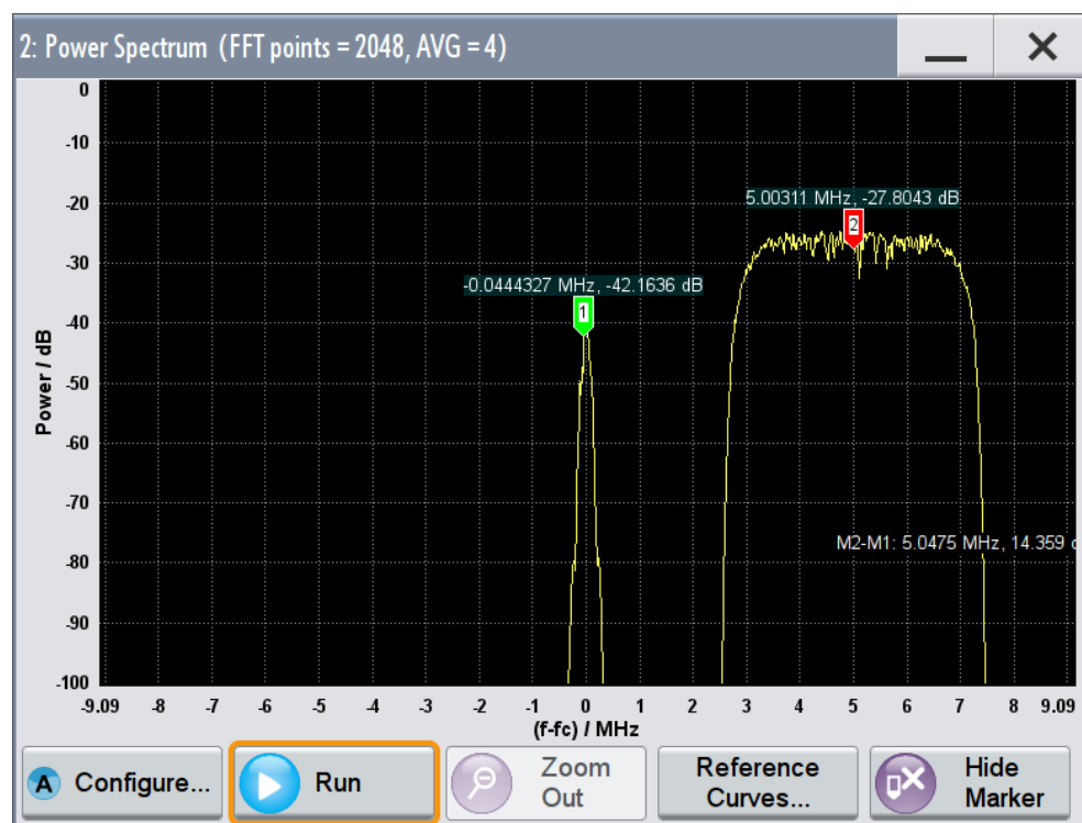
Figure 9-15: Power spectrum with attenuated GSM signal and shifted WCDMA signal
