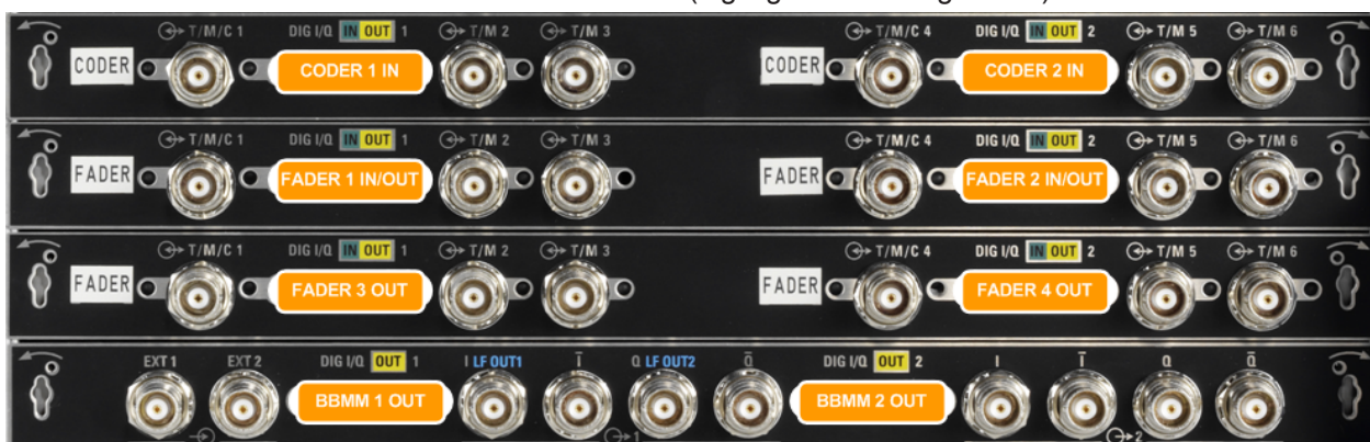
Figure 4-1: Location of the digital input and output interfaces (part view of the rear panel of a fully equipped instrument)
