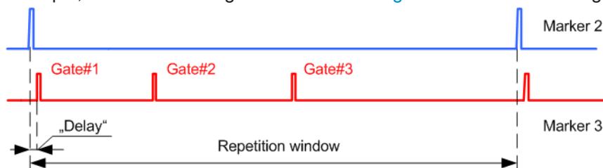
Figure 9-18: Marker signals used in multi-gated acquisition measurement
