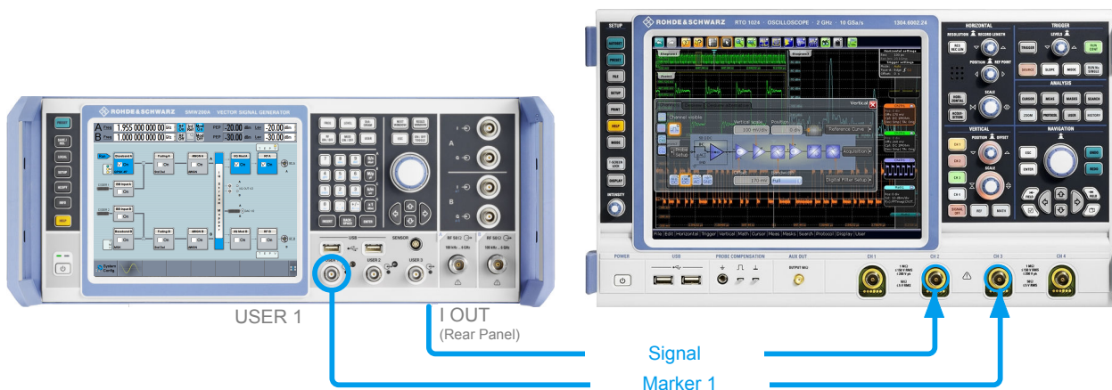
Figure 3-10: Simplified representation of a test setup for signal monitoring**
